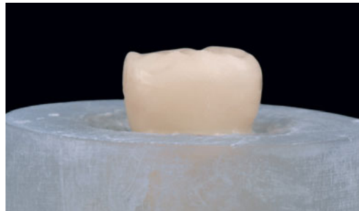
Fig 15 Full Crown Modified Chamfer PIAR after adhesive cementation and before testing. Any marginal adaptation was performed before cementation.
