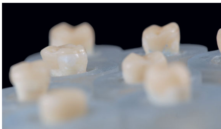
Fig 1 Bonded PIAR samples after thermomechanical loading (TML) and before marginal evaluation.
